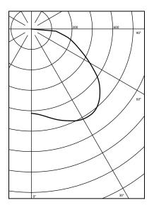
RECESSED 2' X 2' FIXTURE PL1 LENS OPTICS PARALLEL TO LAMP 1-42W BIAX LAMP 73.9% EFFICIENT
