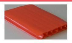
Fluted polypropylene is economical, durable and printable. Corrugated polypropylene sheets are durable use inside and outside, corrugated polypropylene sheet is low in cost, easy to fabricate, and provides good impact resistance.
